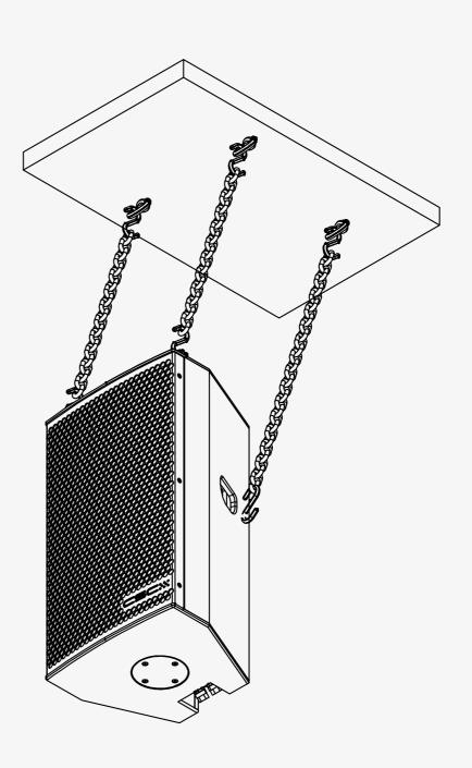
The illustration above displays the Chain Suspension arrangement for the ST 12 Mk2/ ST 12T loudspeaker and identifies the essential hardware supplied.
